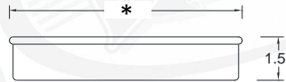
LCNK CANOPY For MULTIPLE FIXTURES *CNK dimensions vary on number of fixtures applied
