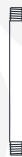
ST(XX) STEM- 1/4" NPT XX = LENGTH OF STEM (EXAMPLE - "ST18" = STEM MOUNT 18" LENGTH)
