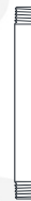
ST(XX) STEM- 1/2" NPT XX = LENGTH OF STEM (EXAMPLE - "ST18" = STEM MOUNT 18" LENGTH)
