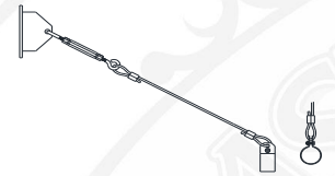
TRB 1/2" - 4' CABLE SUPPORT TRB 3/4" - 4' CABLE SUPPORT
