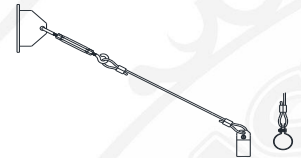
TRB 1/2"-4' Cable SUPPORT TRB 3/4"-4' Cable SUPPORT
