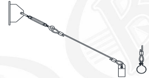
TRB 1/2"-4' Cable SUPPORT TRB 3/4"-4' Cable SUPPORT
