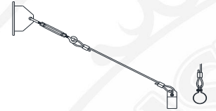
TRB 1/2"-4' Cable SUPPORT TRB 3/4"-4' Cable SUPPORT
