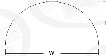
HD10 H-5" W-10" HD12 H-6" W-12" HD14 H-7" W-14" HD16 H-8" W-16" HD18 H-9" W-18" HD20 H-10" W-20" HD24 H-12" W-24" HD30 H-15" W-30" HD36 H-18" W-36" HD42 H-21" W-42" HD48 H-24" W-48"
