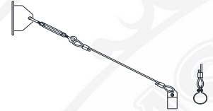
TRB 1/2"-4' Cable SUPPORT TRB 3/4"-4' Cable SUPPORT
