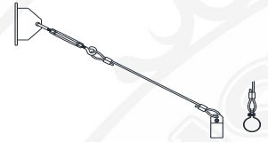
TRB 1/2"-4' Cable SUPPORT TRB 3/4"-4' Cable SUPPORT
