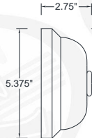
CBC 1/2" 1/2" BACKPLATE COVER CBC 3/4" 3/4" BACKPLATE COVER * Includes slip ring to hold 1/2" or 3/4" arm extension in place
