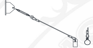
TRB 1/2"-4' Cable SUPPORT TRB 3/4"-4' Cable SUPPORT
