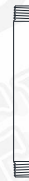
ST(XX) STEM- 1/2" NPT XX = LENGTH OF STEM (EXAMPLE -- "ST18" = STEM MOUNT 18" LENGTH) *CANOPY NOT INCLUDED, ADD IN SECTION D * 1/4" NPT AND 3/4" NPT AVAILABLE UPON REQUEST
