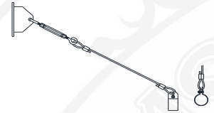
TRB 1/2"-4' Cable SUPPORT TRB 3/4"-4' Cable SUPPORT
