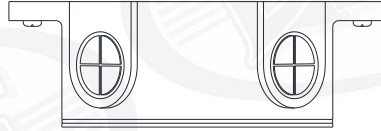
WJB4 1/2 JUNCTION BOX w/ 1/2" KNOCK OUTS WJB4 3/4 JUNCTION BOX w/ 3/4" KNOCK OUTS
