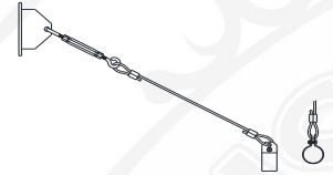
TRB 1/2"-4' Cable SUPPORT TRB 3/4"-4' Cable SUPPORT
