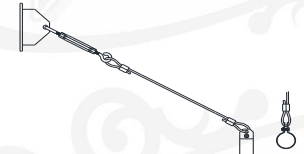
TRB 1/2"-4' Cable SUPPORT TRB 3/4"-4' Cable SUPPORT
