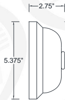
CBC 1/2" 1/2" BACKPLATE COVER CBC 3/4" 3/4" BACKPLATE COVER * Includes slip ring to hold 1/2" or 3/4" arm extension in place
