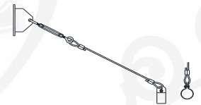
TRB 1/2"-4' Cable SUPPORT TRB 3/4"-4' Cable SUPPORT
