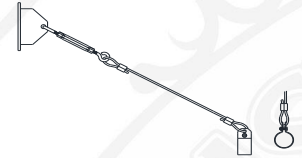
TRB 1/2"-4' Cable SUPPORT TRB 3/4"-4' Cable SUPPORT
