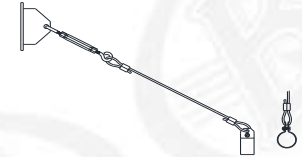
TRB 1/2"-4' Cable SUPPORT TRB 3/4"-4' Cable SUPPORT
