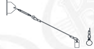
TRB 1/2"-4' Cable SUPPORT TRB 3/4"-4' Cable SUPPORT
